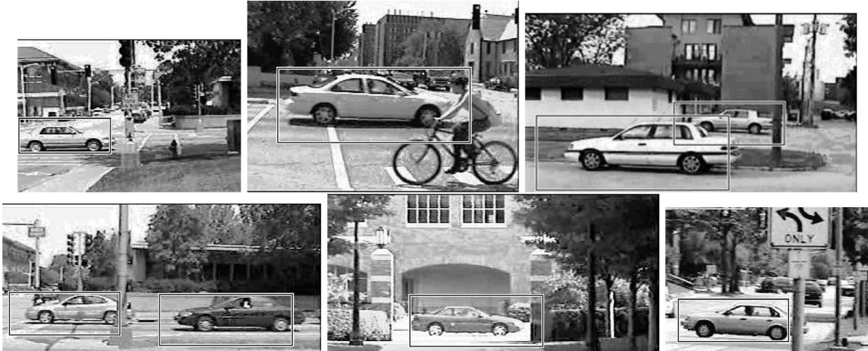
Fig. 14. Examples of test images on which our multiscale detection system achieved perfect detection results. Results shown are with the neighborhood suppression algorithm (see Section 2.4) at the point of highest F-measure from Table 4, i.e., using an activation threshold of 0.95. The windows are drawn by a separate evaluator program at the exact locations and scales output by the detector.
