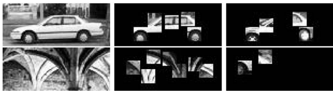
Fig. 4. Examples of the part detection process applied to a positive image (top row) and a negative image (bottom row) during training. Center images show the patches highlighted by the interest operator; notice how this successfully captures the interesting regions in the image. These highlighted interest patches are then matched with vocabulary parts. In the right images, the highlighted patches are replaced by an arbitrary member of the part cluster (if any) matched by this detection process. These parts, together with the spatial relations among them, form our representation of the image.
